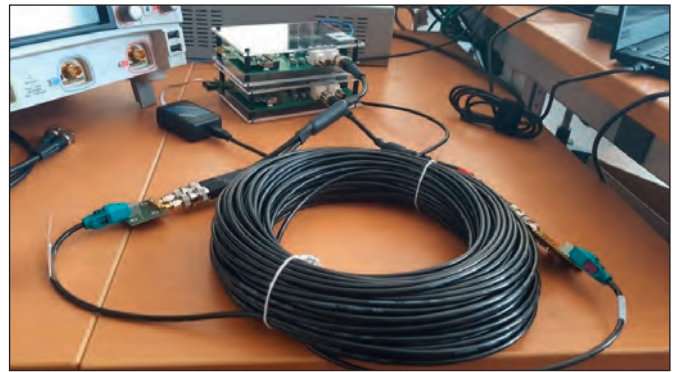
Figure 3: Measurements with OFDM Physical Layer combined with a 50 m reduced twisted pair cable
